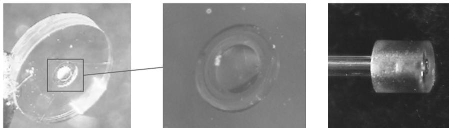
Figure 1. Hemi-aspheric optical concentrator diamond-turned from PEI disc (left) and detail view (center); PEI molded optical insert (right) having integrated concentrator and fiber alignment bore, with POF installed.
