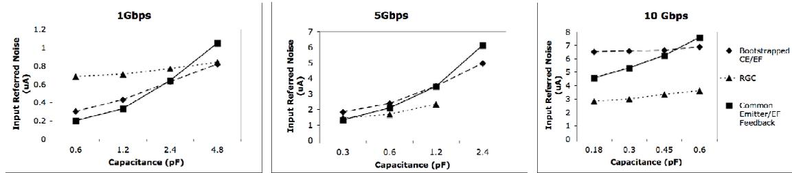
Figure 4. The scaling of input referred noise with photodiode capacitance for the CE/EF (square/solid line), RGC (triangle/dotted line), and bootstrapped CE/EF (diamond/dashed line) for three different bit rates: 1, 5, and 10 Gbps
