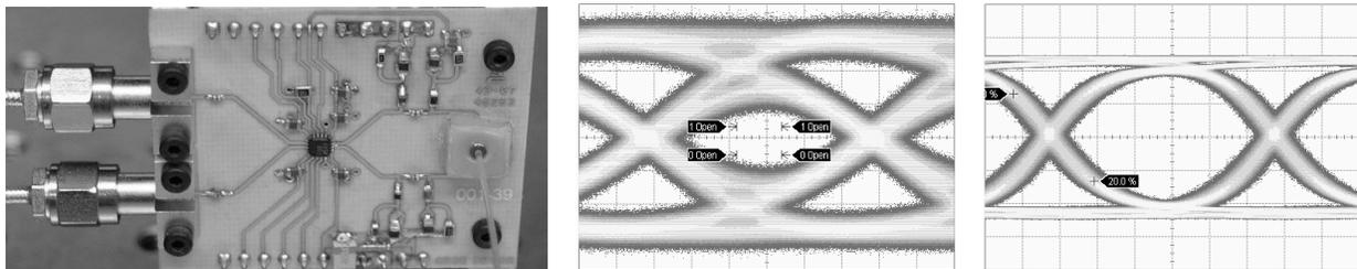
Figure 5. COB transmitter with encapsulated insert (left); Eye diagram for 200 meters of GI-POF (center); Eye diagram for 1 meter (right).
