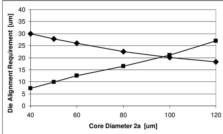
Figure 2. Die-referred alignment requirement to meet a 0.5 dB loss criterion; (■) Tx with 75% fill factor; (◆) Rx with 80  $\mu\text{m}$  diameter detector.
