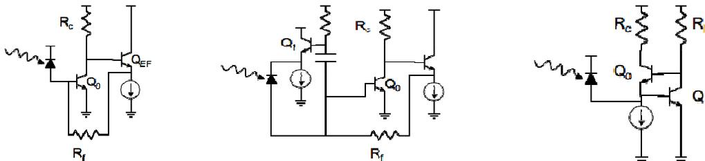
Figure 3. The CE/EF circuit (left), the bootstrapped CE/EF (middle), and the RGC (right)
