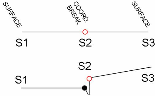
Figure 3. Coordinate break (red circle) between optical axes, before and after transformation: First decenter X, then decenter Y, then tilt about the X-axis, tilt about the Y-axis, and finally, tilt about the Z-axis.
