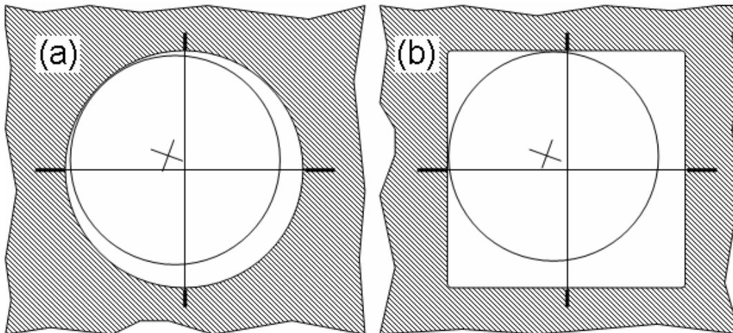
Figure 6. Actual (a) and simulated (b) model of fiber in bore showing overestimation of decentering value.
