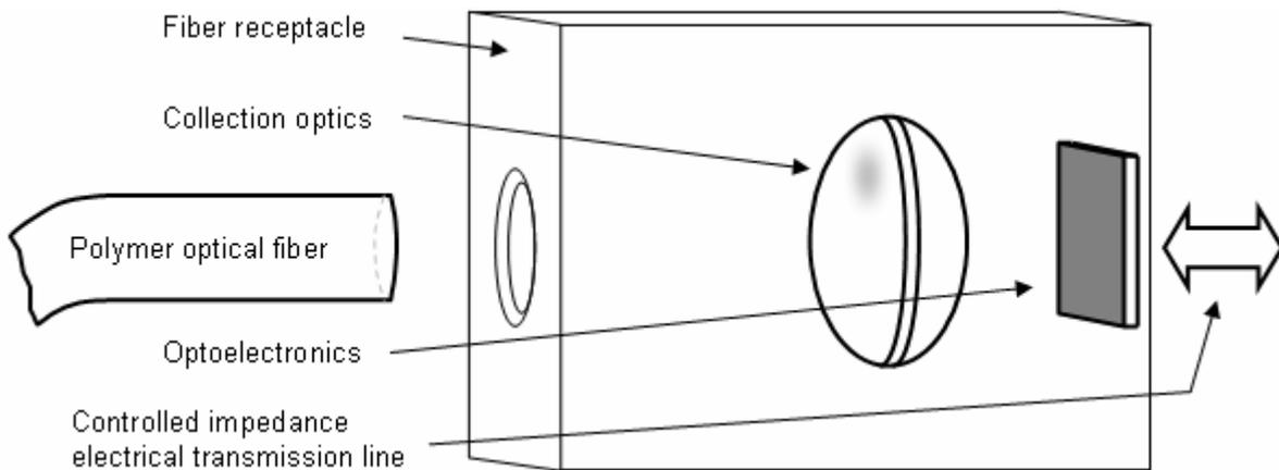
Figure 1. Block diagram of TOSA or ROSA showing major components, and uninstalled POF. Receptacle bore and fiber retention mechanism is not shown for clarity. In the drawing light would propagate from fiber-to-detector for a ROSA, and right-to-left for a TOSA.
