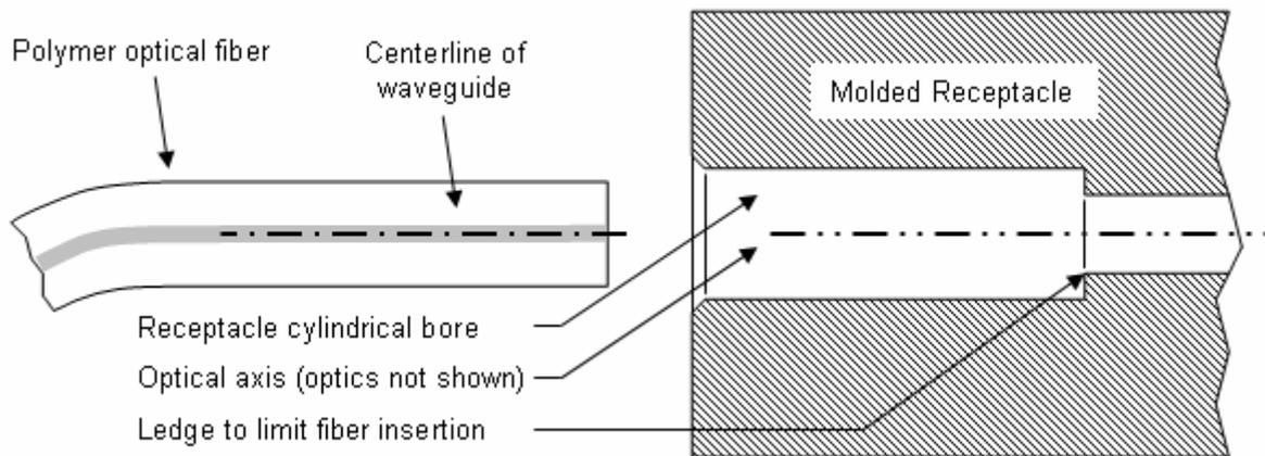
Figure 2. Cross-sectional side view of the optical fiber receptacle showing the two cylindrical counterbores used to mechanically align the fiber waveguide with respect to the collection optics (not shown).
