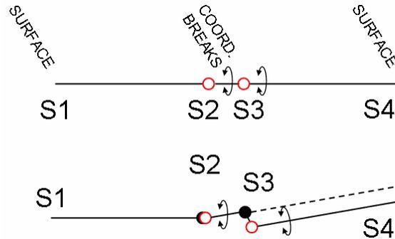
Figure 7. Improved dual coordinate break in optical axis, before and after: First decenter X only, then rotate  $\pm 180^\circ$  about the Z axis. A second coordinate break at zero distance then tilts about the Y axis only, followed by another  $\pm 180^\circ$  about Z.
