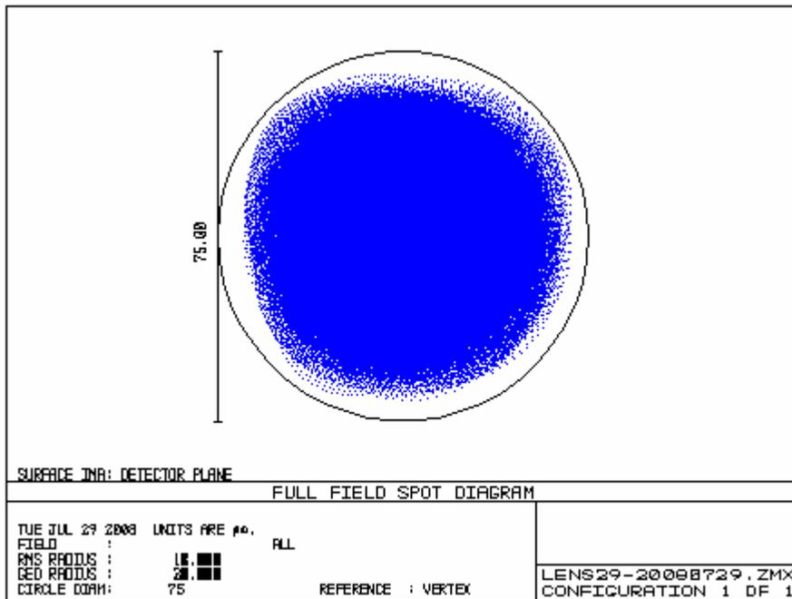
Figure 5. Geometric full field spot diagram for 100 Monte Carlo runs. Note the non circular shape.
