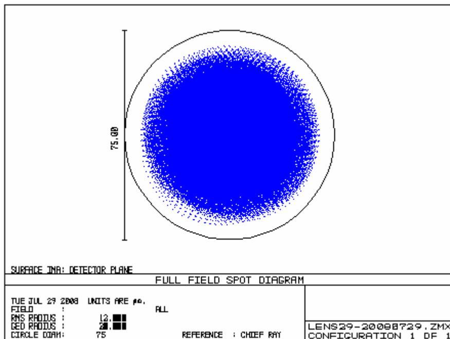
Figure 8. Geometric full field spot diagram for 100 Monte Carlo runs.
