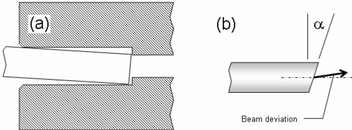
Figure 4 (a) illustration of fiber tilting in bore (b) effect of refraction with non-perpendicular POF endface.
