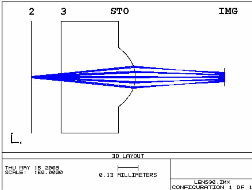
Figure 2. Layout of optical concentrator within the insert showing the object (coincident with surface 2). For the same reason the coordinate breaks are not visible in this layout but are coincident with the object and image planes.
