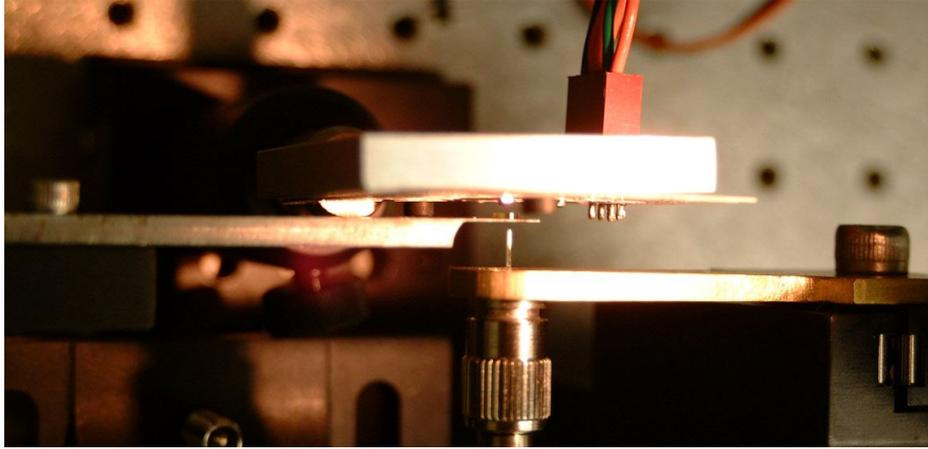
Figure 6. Top view of test setup for COB showing the edge of the PCB, the prototype collection optics and the POF.
