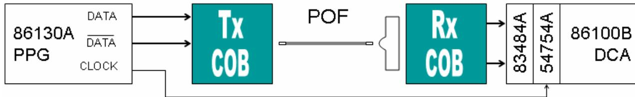
Figure 8. Block diagram of the COB transmitter and link test setup.
