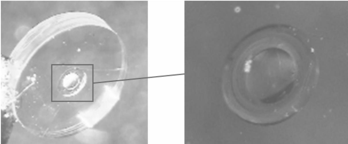
Figure 4. Photograph of diamond-turned polyetherimide (PEI) optical concentrator with detail of aspheric surface.
