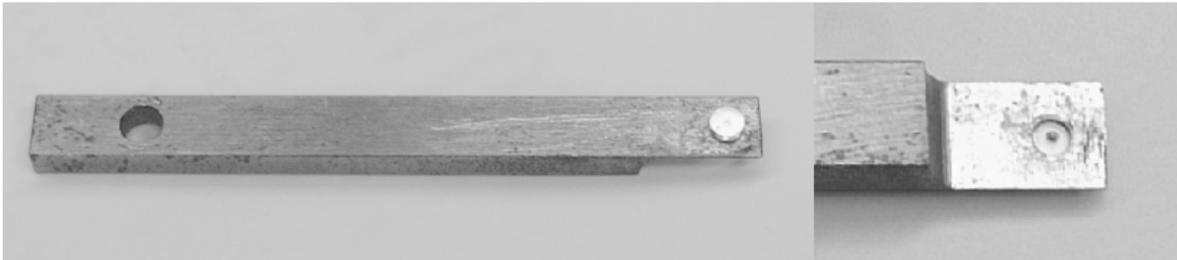
Figure 5. Photograph of blade and mounted diamond-turned prototype from planar side (L) and curved side (R).
