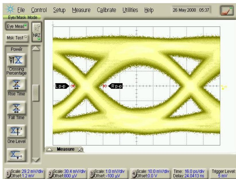
Figure 9. Eye diagram for Rx COB with reference transmitter operating at 10 Gbps for 30 hrs.
