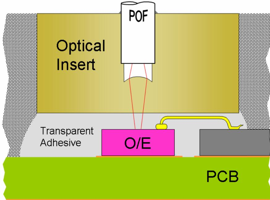
Figure 1. Cross-section of optical insert with optoelectronic die, wirebonding, and silicon die. The optical insert contains the alignment features for the fiber, an air gap, and the non-imaging optical concentrator.
