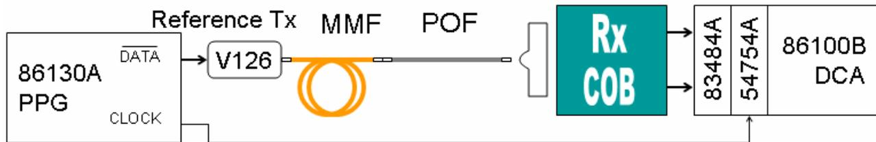
Figure 7. Block diagram of the COB receiver test setup. A pulse pattern generator (PPG) is the signal source and the digital communications analyzer (DCA) is used to characterize the Rx performance.
