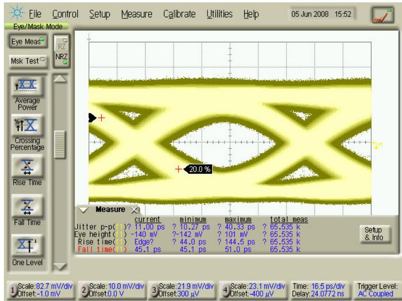
Figure 10. Eye diagram for 10 m POF link operating at 10 Gbps for 30 hrs.
