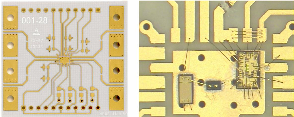
Figure 3. Photograph of 40 mm x 40 mm substrate for COB and magnified view die attach pad populated with commercial optoelectronic and electronic dice. The central die is a GaAs PIN photodiode, the left component is a 180 pF chip bypass capacitor, and the IC on the right is a commercially available transimpedance amplifier.
