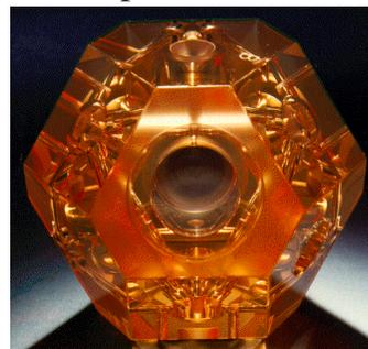
Monolithic Ring Laser Gyro (MRLG). Copyright © 2006 Kearfott Guidance and Navigation Corporation. Reproduced with permission.
