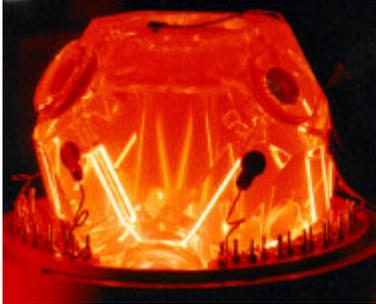
Monolithic Ring Laser Gyro (MRLG). Copyright © 2000 Konforfit Guidance and Navigation Corporation. Reproduced with permission.
