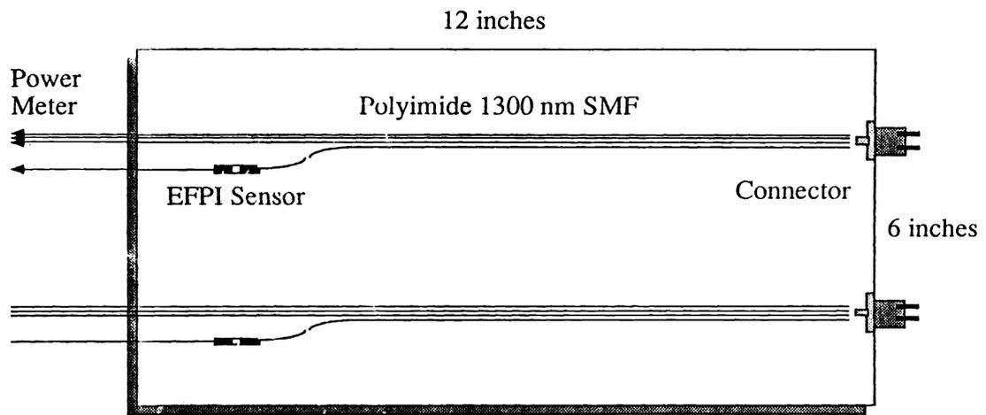
**Figure 2.** Optical fiber and fiber sensor layout configuration.
