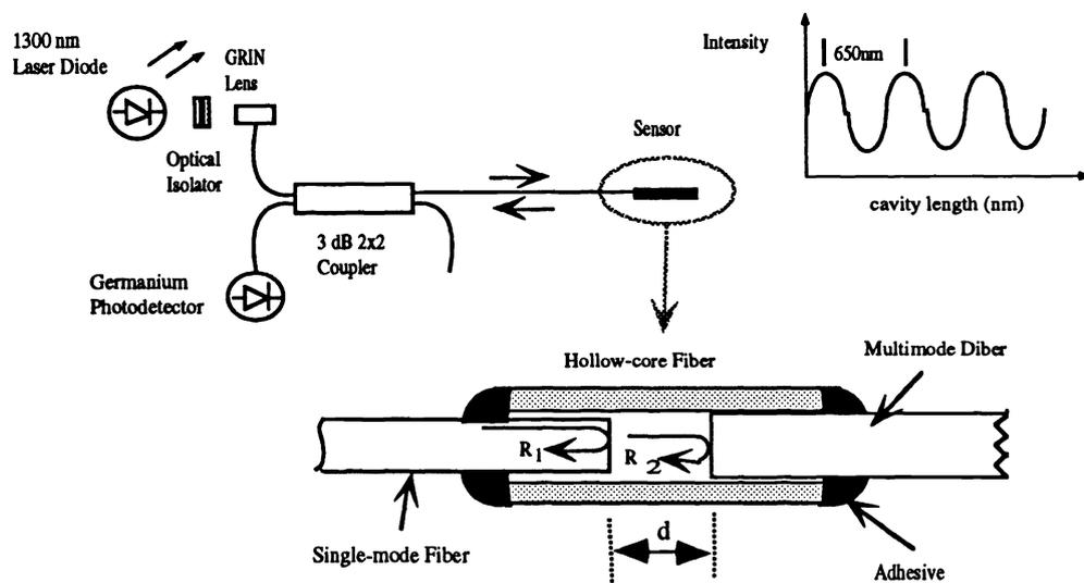
**Figure 4.** Extrinsic Fabry-Perot interferometric fiber sensor.
