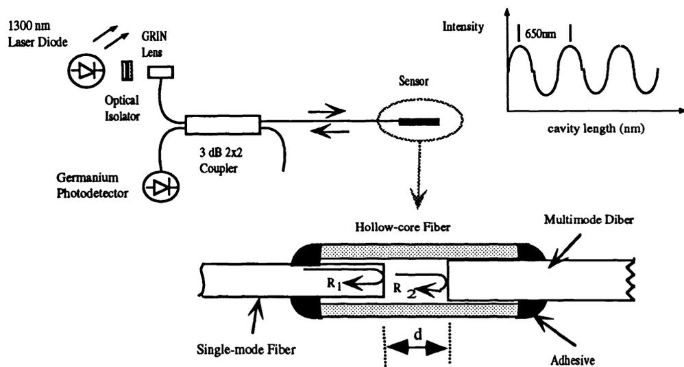
**Figure 4.** Extrinsic Fabry-Perot interferometric fiber sensor.
