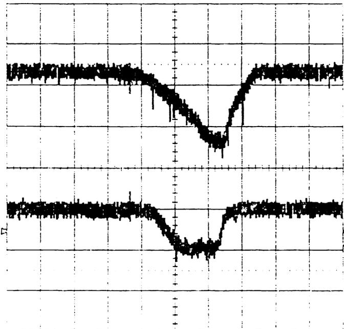
**Figure 7.** EFPI output under loading conditions, showing successful connectorization of embedded fiber sensors, a) EFPI output during bending through connector 1 and b) EFPI output from connector 2. Both oscilloscope traces are 1 volt/div vertical scale and 1 sec/div horizontal scale.
