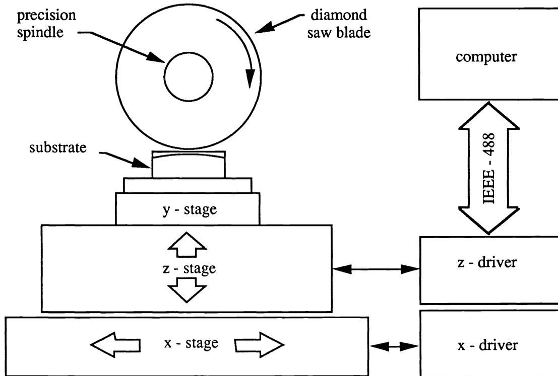
Figure 1. Computer-controlled groove generator.
