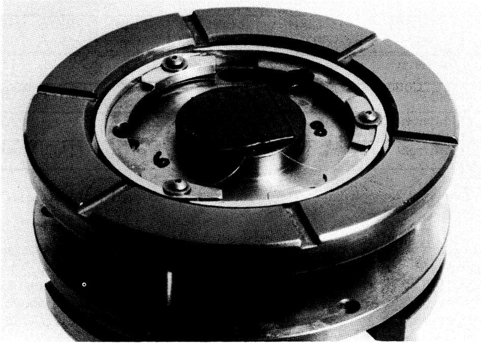
Figure 3. Face of polishing jig showing conditioning ring and substrates.
