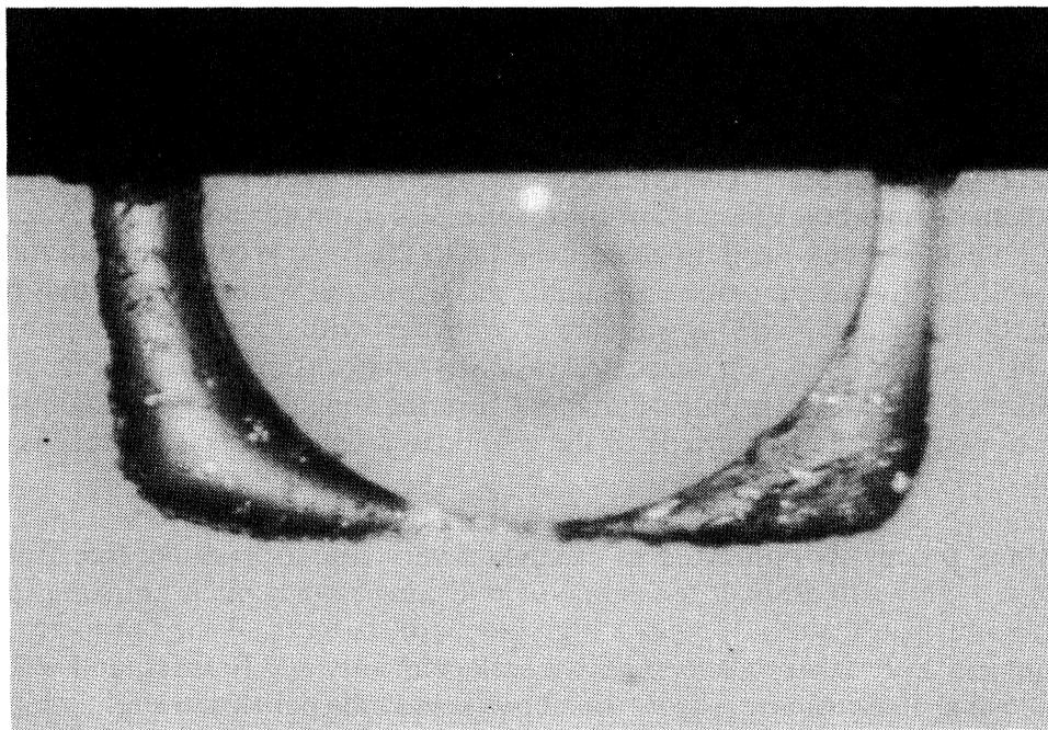
Figure 2. Groove and polished PANDA fiber cross section.
