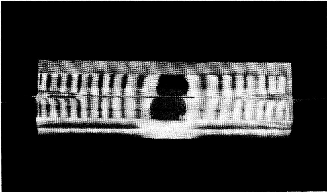
Figure 4. Coupler with incomplete optical contact bond.
