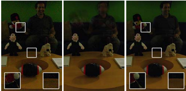
Figure 6. Stack consisting of 10 pictures affected by ISO noise, one of which is shown on the left. The noise can be attenuated by averaging the pixel values across the stack, but moving objects can cause ghosting as shown in the middle picture. Alternatively, a reference picture can be selected and only pixels consistent with it can be averaged together as shown in the picture on the right. Note that, where movement occurs, noise may be not removed (see inset on the puppet).
