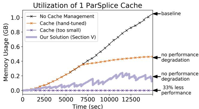
Figure 1: Using our data management language and policy engine, we design a dynamically sized caching policy (thick line) for ParSplice. Compared to existing configurations (thin lines with  $\times$ 's), our solution saves the most memory without sacrificing performance and works for a variety of inputs. Solutions labeled “no performance degradation” are in comparison to the baseline of a cache of unlimited size.
