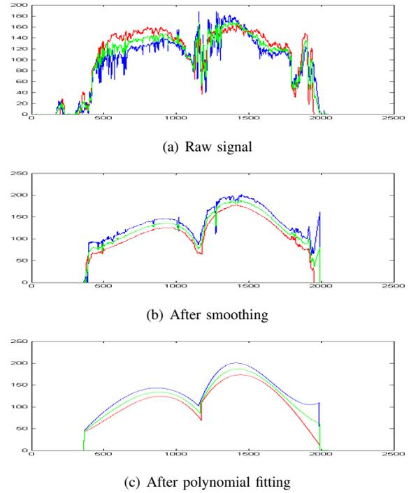
Figure 5. Depth profiles before and after smoothing
