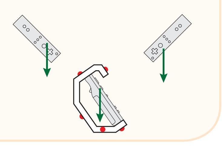
In cases where the previous state is known, a simple gradientdescent solve is performed. The Wii Remote returns data at 100Hz, so the change between two adjacent frames is small enough that local minima are rarely found. If GD does get stuck in a local minima, the first approach is used.
