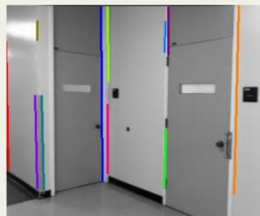
Identified pairs of parallel lines oriented along one canonical directions
