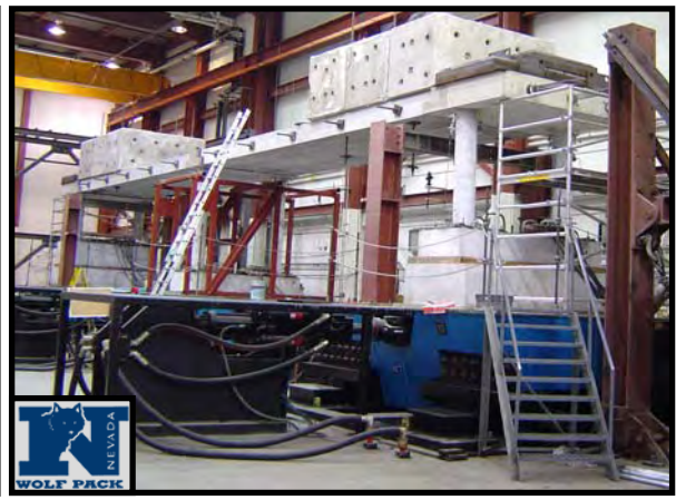
Figure 3: Photograph of bridge model set-up on shake tables at the University of Nevada, Reno. (After Johnson et al., 2006)
