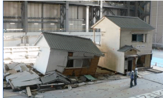
Photo 1 A pair of thirty-years old wooden houses, one with retrofit (survived) and the other without (failed).
