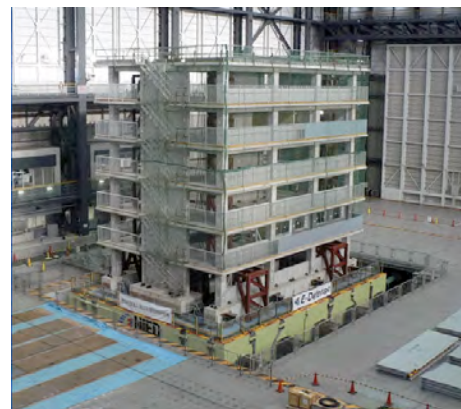
Photo 2 A six-story RC wall-frame (1,000 metric ton), subjected to 1995 JMA Kobe in all three directions
