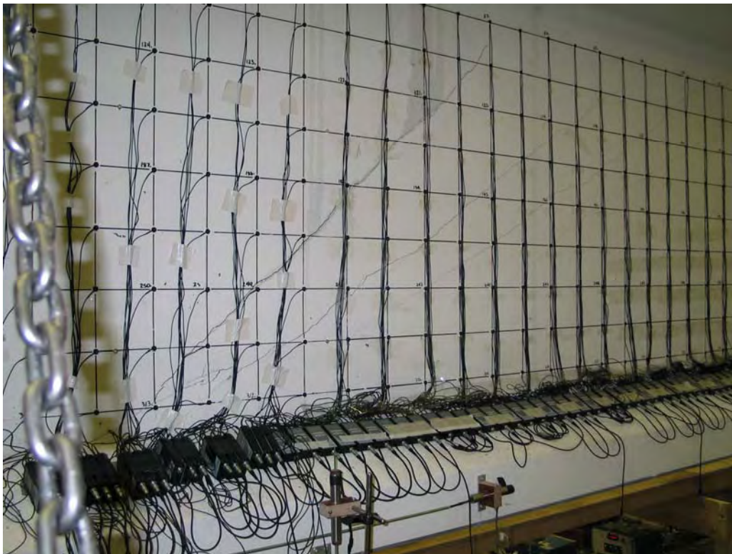
Figure 3: Distribution of Krypton LED Targets in Grid on Test Structure
