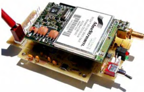
Figure 1. Fully assembled wireless sensing unit prototype developed at the University of Michigan by Professor Jerry Lynch (battery and external container not shown for clarity).
